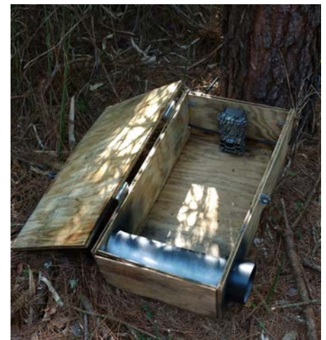
"Mostela" camera trap used in the pilot camera survey of weasels (NCWRC)
